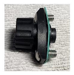
**5.** To ensure that the adjuster is correctly orientated on the shock absorber, check that when the adjuster is rotated full anticlockwise, the adjusting pin is not protruding.
