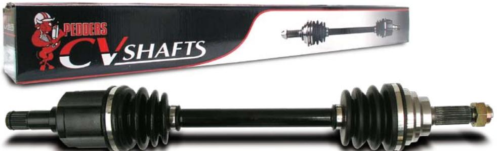
CV joints are protected from contamination by air tight rubber boots secured with metal retaining clips. Failure of these boots is the primary reason for CV joint failure. A split or broken boot will eventually cause the failure of the CV joint in all cases.
