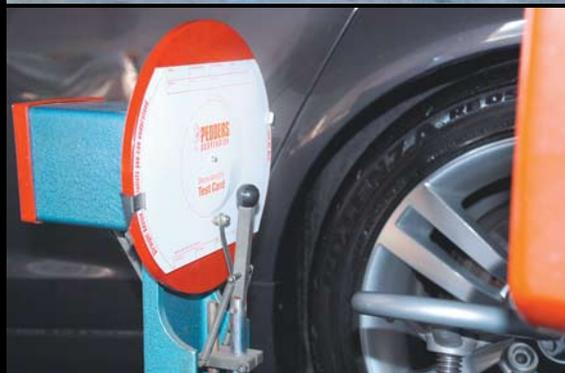
How well your car passes this test will be determined by the difference between each shock's maximum figure value, obtained during the test and a known standard: A Pedders shock absorber unit.
