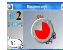
**Axle Weight Test\*:** The test lane measures the front and rear axle weight of the vehicle. This information is vital for checking to see if the vehicle weight falls within its gross vehicle mass (G.V.M.) which is ideal information for people who use their vehicle to carry heavy loads or tow regularly.
