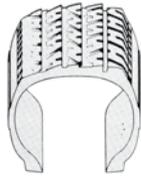
**Feathering:** This is caused by erratic scrubbing against the road when the tyre is in need of toe-in or toe-out alignment correction.
