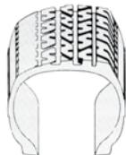
**One-side wear:** Here's another type of alignment problem; excessive camber, which means that the tyre is leaning too much to the inside or outside of the tread, and placing all work on one side of tire.
