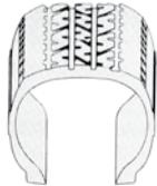
**Under-inflation:** When a tyre is underinflated, most of its contact with the road is on the outer tread rib, or shoulder, causing faster wear here than in the middle. Be sure to check the tyre's air pressure.
