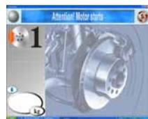
**Brake Force Test:** The brake force test uses dynamic rollers to check the braking system. This test measures brake force on each wheel individually to assess if there is any variation in effectiveness for the service and park brake systems.
