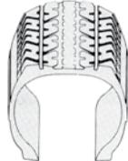
**Over-inflation:** This can cause premature wear in the centre of the treaded area of the tyre, as the centre of the foot print is in contact with the road surface more that it was designed for.
