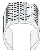
**Cupping:** This means the car may need wheels balanced, or new shock absorbers or ball joints, or both.
